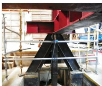
Point Load Test Setup
