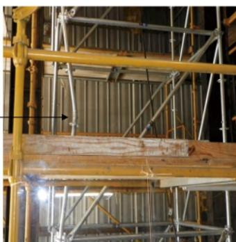
Typical deflection of leg at failure
