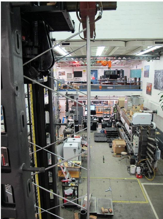
Before test (#1: 5' X 19' scaffold assembly)
